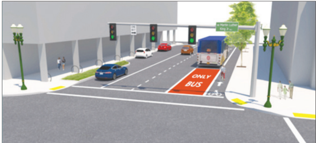
A rendering of the red bus-and-turn (BAT) lane the Portland Bureau of Transportation will install on East Burnside Street between Martin Luther King Jr. Boulevard and 12th Avenue. (PBOT)
