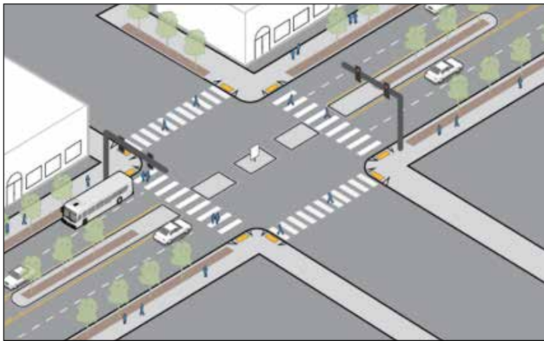
Illustration of changes proposed on Northeast Martin Luther King Boulevard at Mason Street, where concrete barriers in the intersection will allow pedestrians and bikes to cross on Mason Street, while restricting motor vehicles to right-turns. (PBOT)
