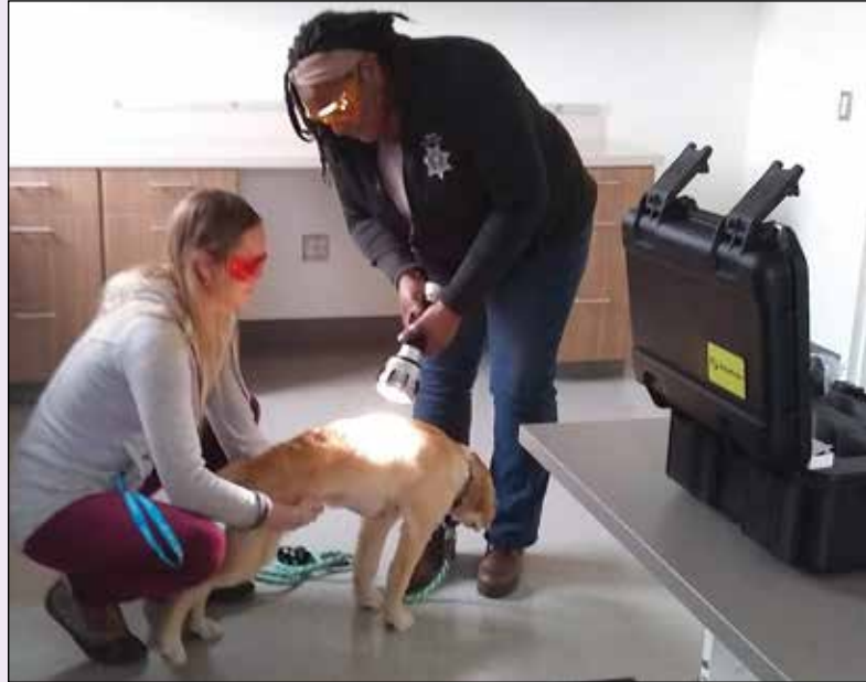
Forensics coordinator Samantha Lee (left) and support specialist and evidence technician Lila Obeng demonstrate the use of an alternate light source to look for evidence such as fluids and fibers not visible using typical light wavelengths. (Lisa Lakes)
